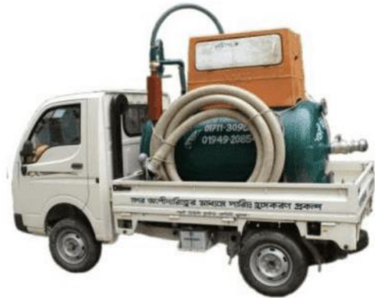
Figure 6.2: Vacutug for desludging Pit/ Septic tank
