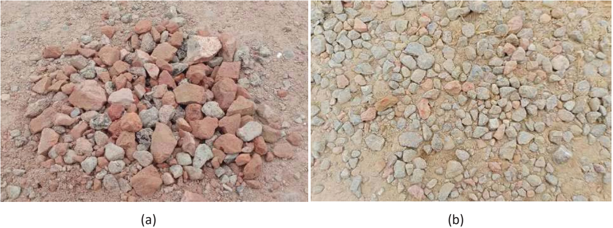
Figure 3: Aggregate collected from sub-base of strengthened road
