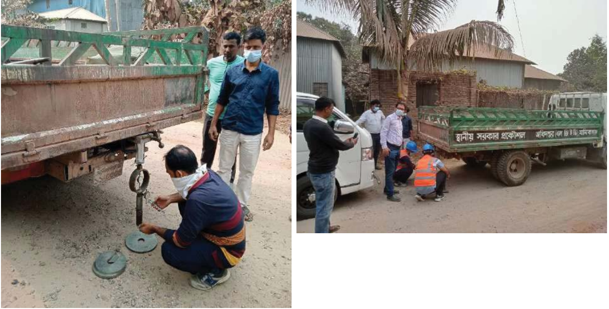
Figure 15: Field CBR Test by BUET Team
