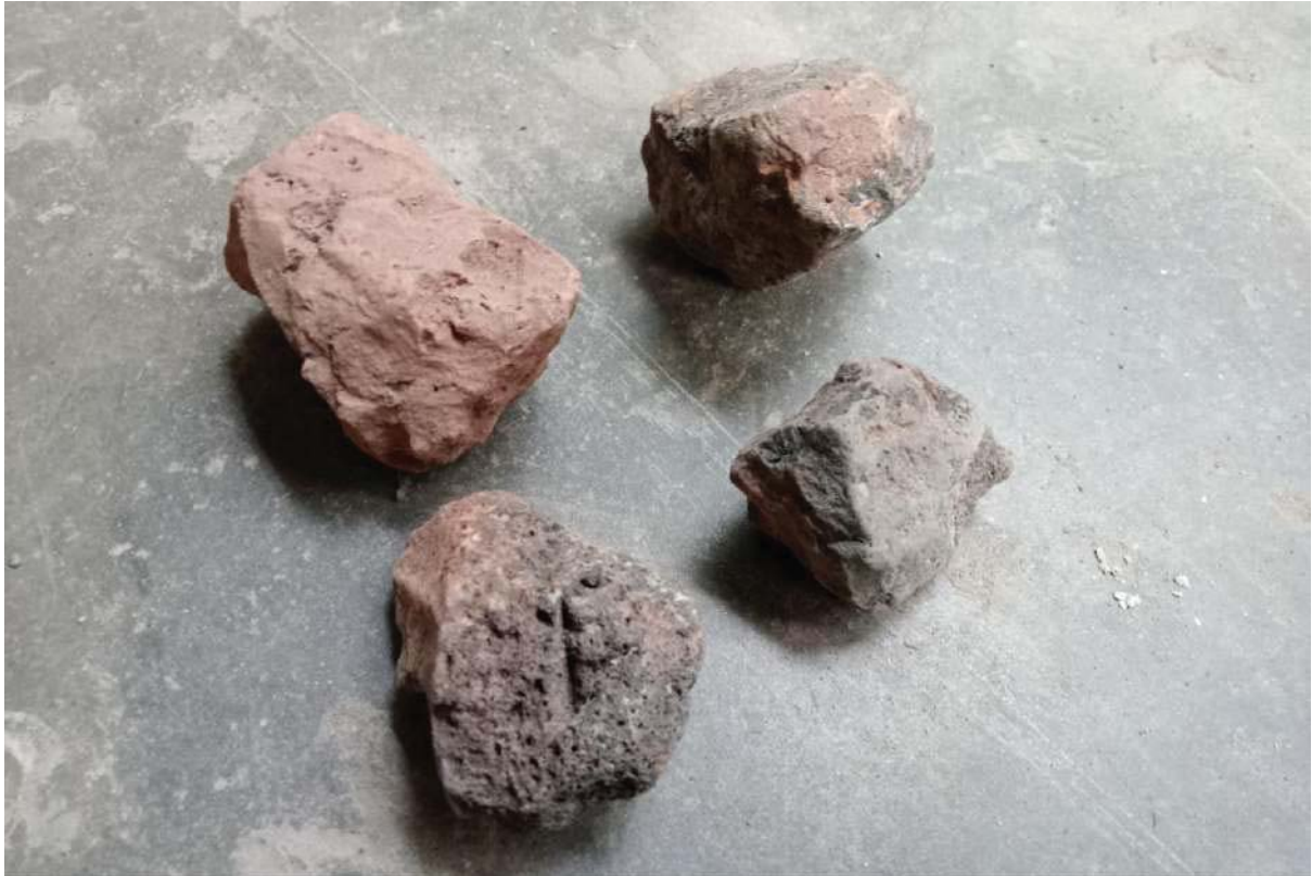
Figure 7: Greater than 1" Size RBCA (Picked Jhama Brick Aggregate)
