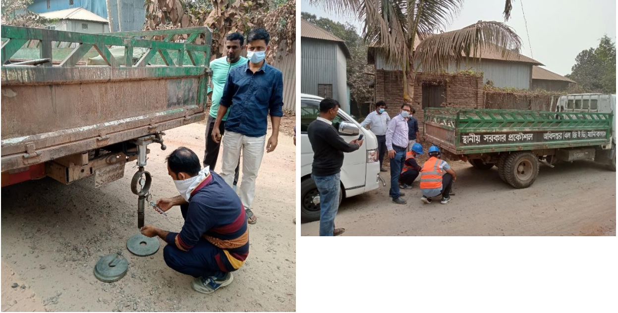
Figure 16: Field CBR Test by BUET Team
