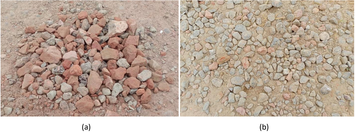
Figure 3: Aggregate collected from sub-base of strengthened road
