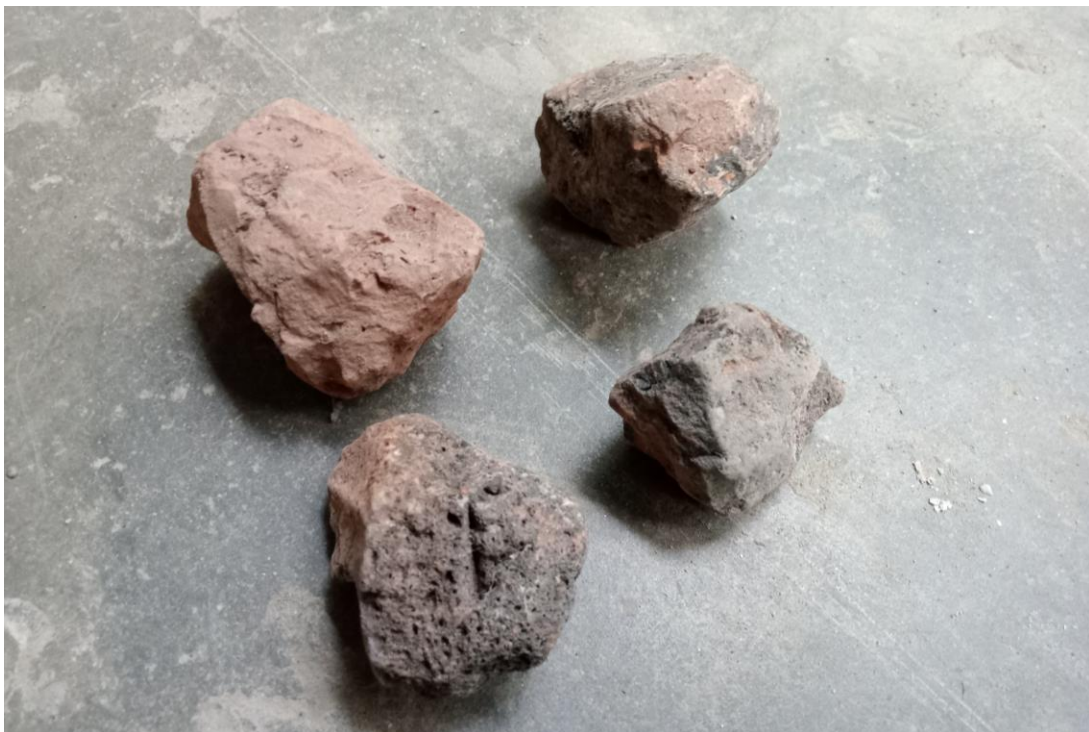
Figure 8: Greater than 1" Size RBCA (Picked Jhama Brick Aggregate)
