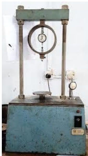
Figure 19: Marshall Stability Test Apparatus
