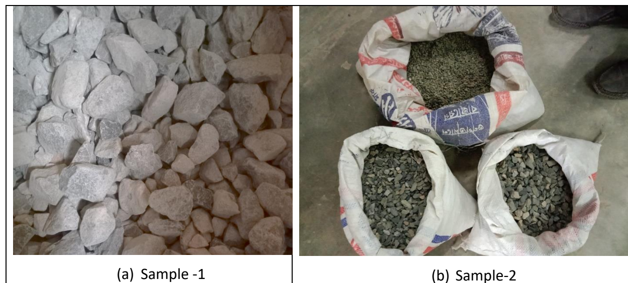
Figure 23: Picture of Virgin Aggregate Samples Supplied by LGED for Marshall Mix Design
