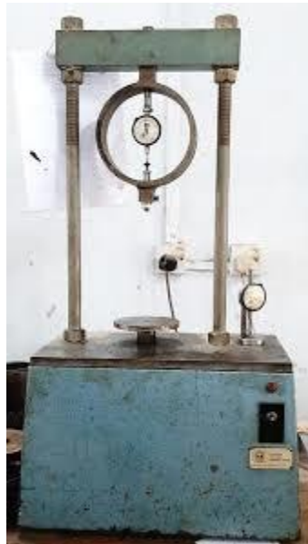
Figure 5: Marshall Stability Test Apparatus
