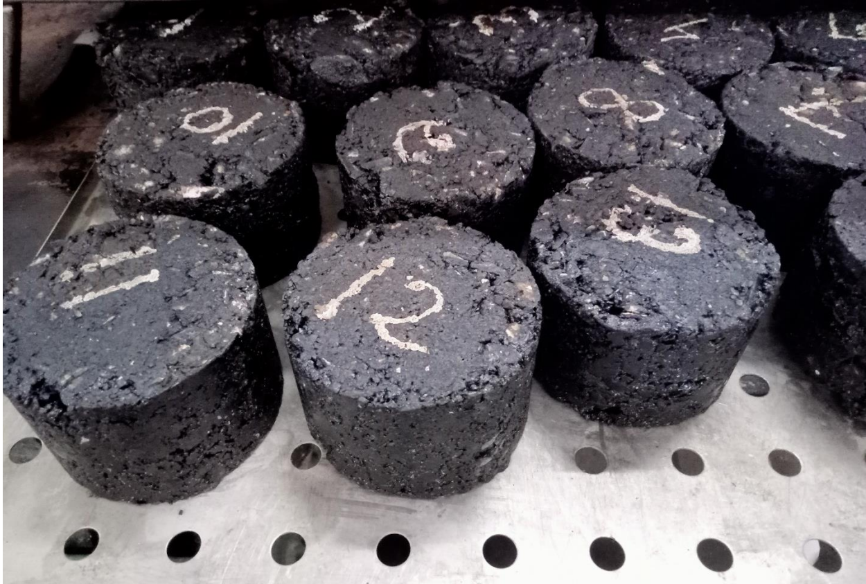
Figure 10: Marshall Mix Design Samples in Laboratory.
