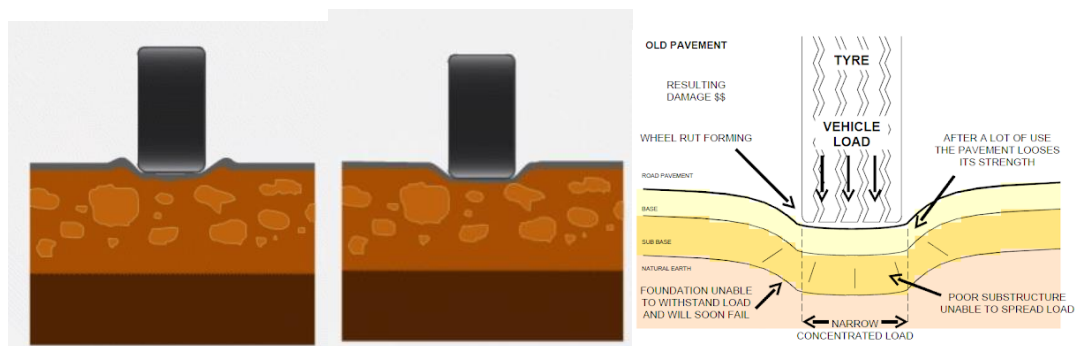
Left: Plastic deformation of the asphalt layer. Centre: Simple depression without rutting. Right: Pathology formation process
